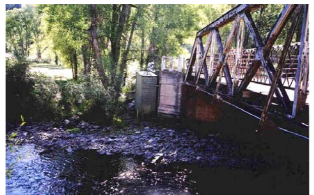
Figure 2-2: USGS Gage at the Montelores Bridge downstream of Rico at the County Line.
